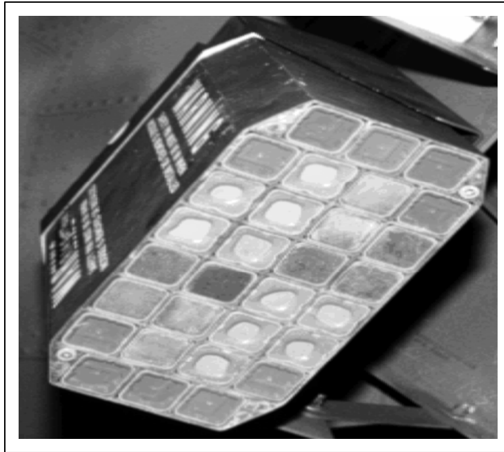
Figure D-7. AN/ALE-47 counter measures dispenser system
